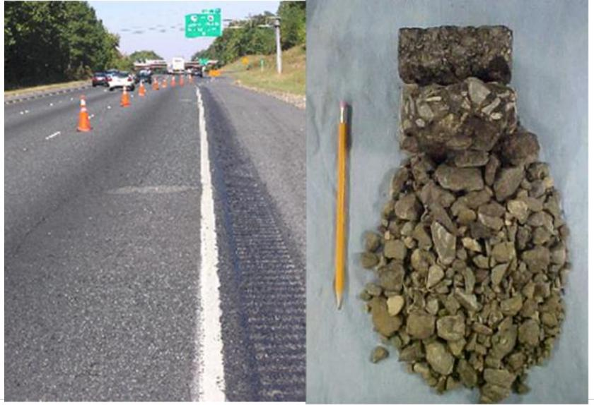
The service life of SM in this corridor of 195 was down to Six Years – After FWD and coring selected on the "Base Damage Index" Severely stripped base mix layers were found at re-occurring intervals. BM was placed in the 1980's How about SMA - "constituents" should be interpreted to mean asphalt binder, aggregates, and air voids
